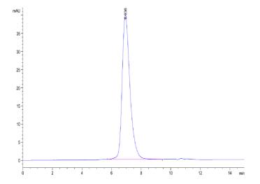
The purity of Biotinylated Human CD155 (Primary Amine Labeling) is greater than 95% as determined by SEC-HPLC.
